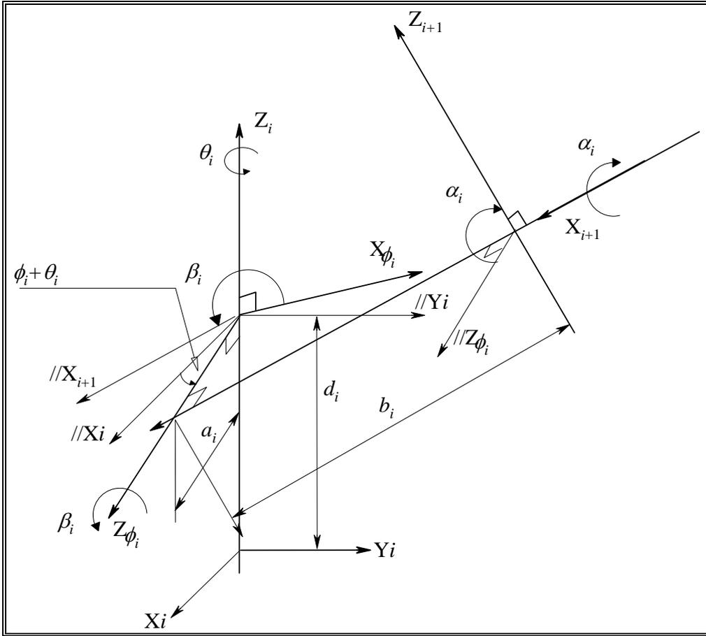
Figure (1): The Kinematic Notation of the  $\phi$ -Model.
