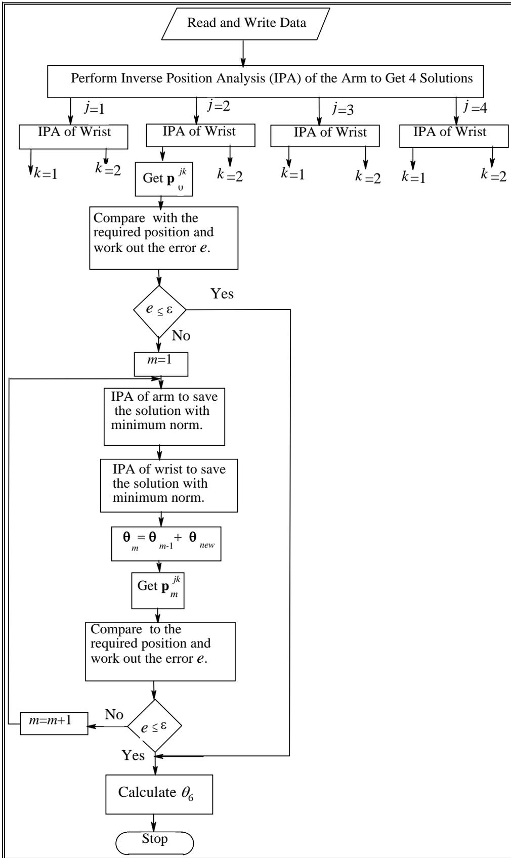
Figure (4): Inverse Position Analysis of Robots Using Elementary Motions.
