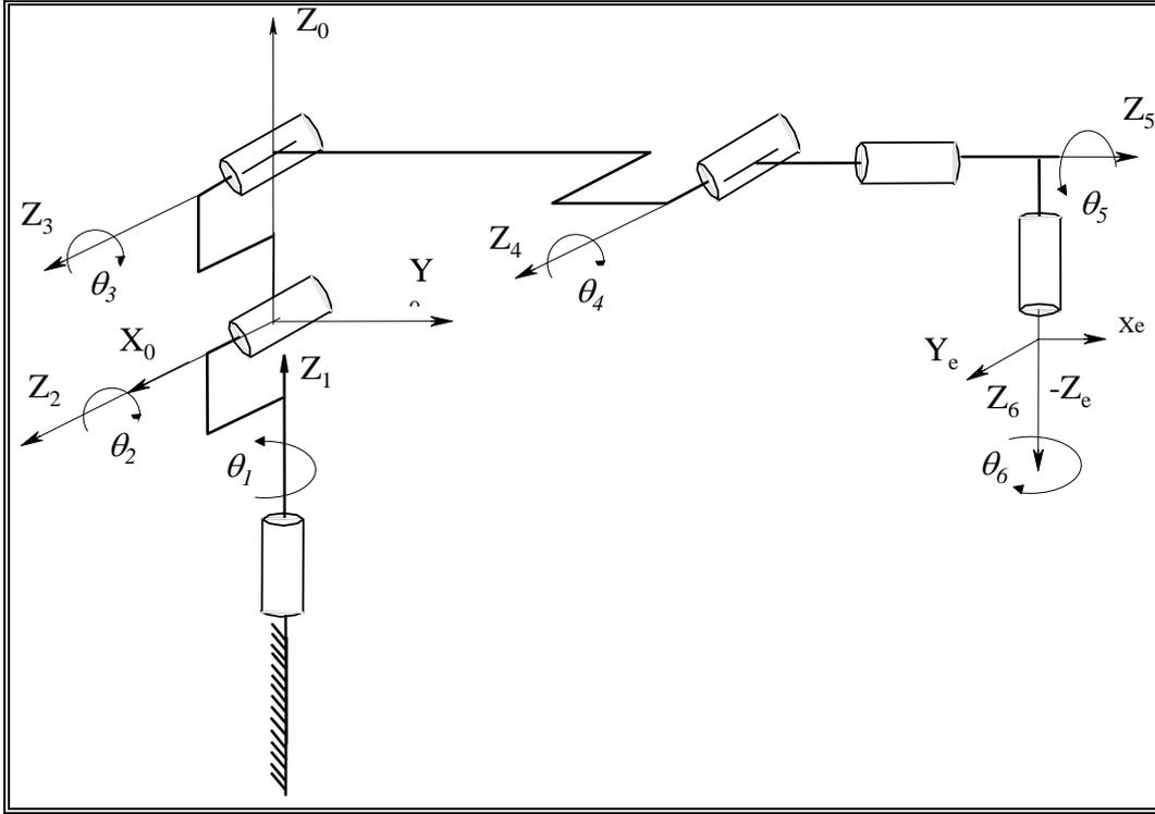
Figure (5): Schematic Diagram of the Robot Used for Experimental Verification.
