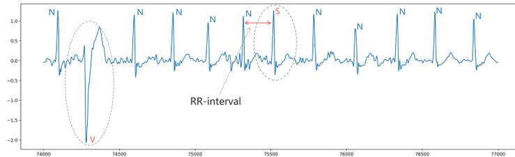
**Fig. 1.** A sample ECG recording that contains  $N$ ,  $S$  and  $V$  heartbeats. Note:  $RR$ -intervals denote the time distance between two successive  $R$  peaks.
