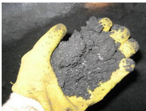
Fig 2. Thermally fragmented rock [4]
