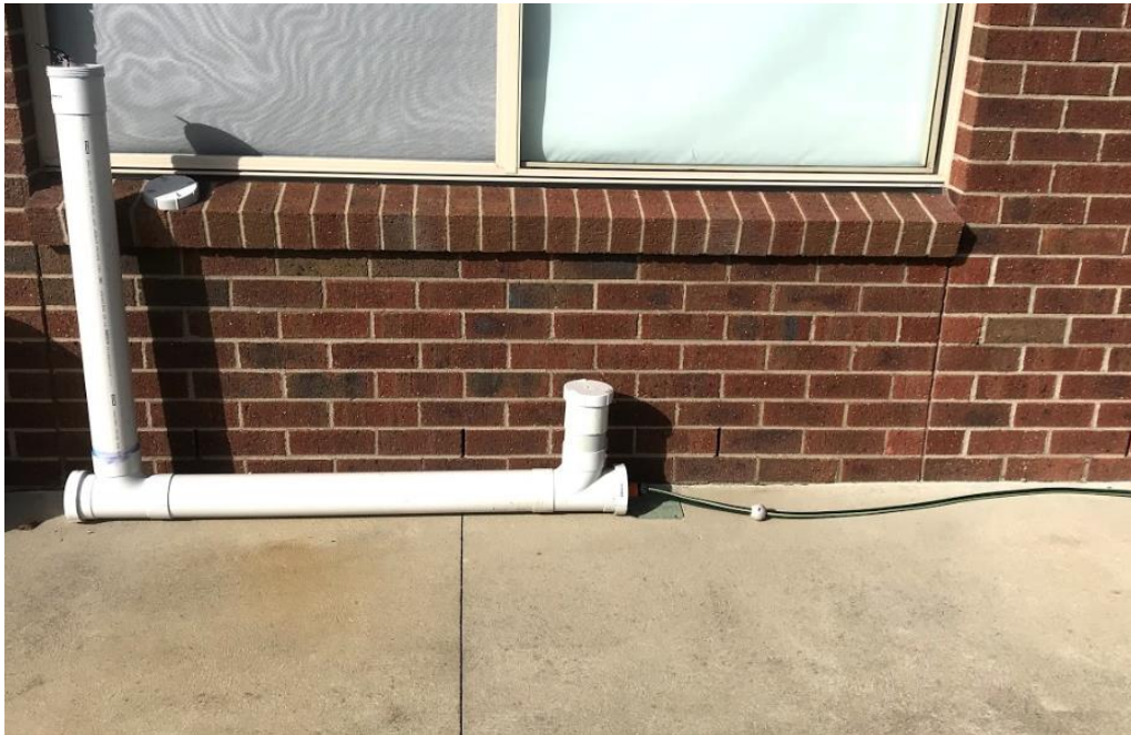
Figure 4-19: The test bed being filled with water. A standard garden hose is attached to the fitting and turned on, allowing water to fill the pipe. Our mote can be seen at the top of the tall pipe.
