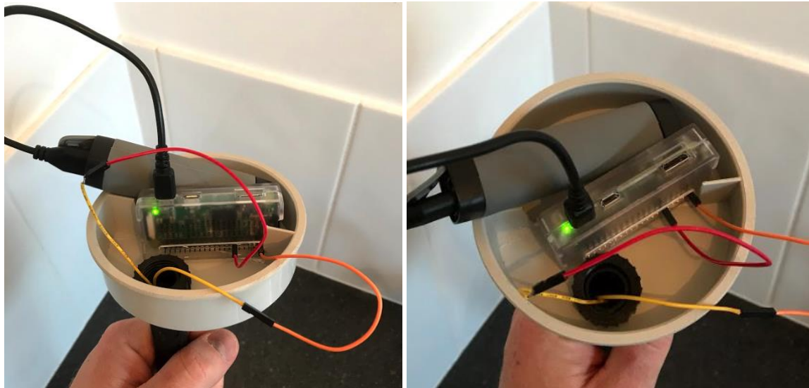
Figure 4-18: The mote placed inside our custom pipe cap. Unfortunately, as the USB battery we utilised was too large to properly fit inside the pipe cap, the mote system protruded from the cap. However, as this device is only a prototype, we were less concerned with the relative size and more with ensuring the device had power. Dedicated, small batteries are available for our purpose, however we were unable to procure one in time for testing.
