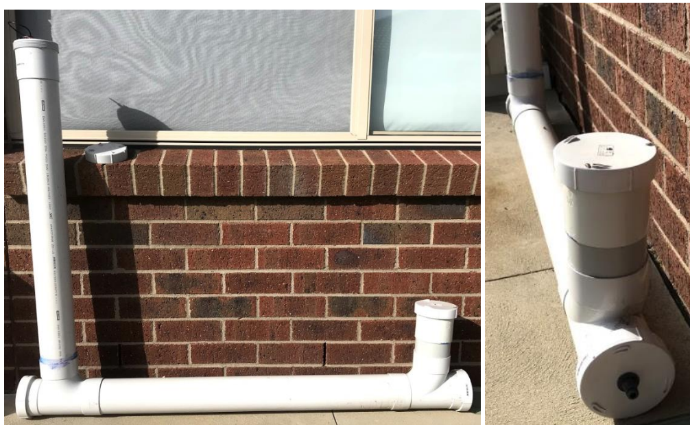
Figure 4-15: Photographs of the completed test bed from varying perspectives. Aside from an additional, shorter perpendicular pipe, this confirms to the general design laid down in the previous figure. All components specified in the design are shown in the left image, while the right image has been added to show the hose fitting for allowing water in. When water is introduced with that hose fitting, the perpendicular pipes will begin to fill with water. The mote will be placed in the tall pipe in the left image, and the float switch will activate when the rising surface reaches it.
