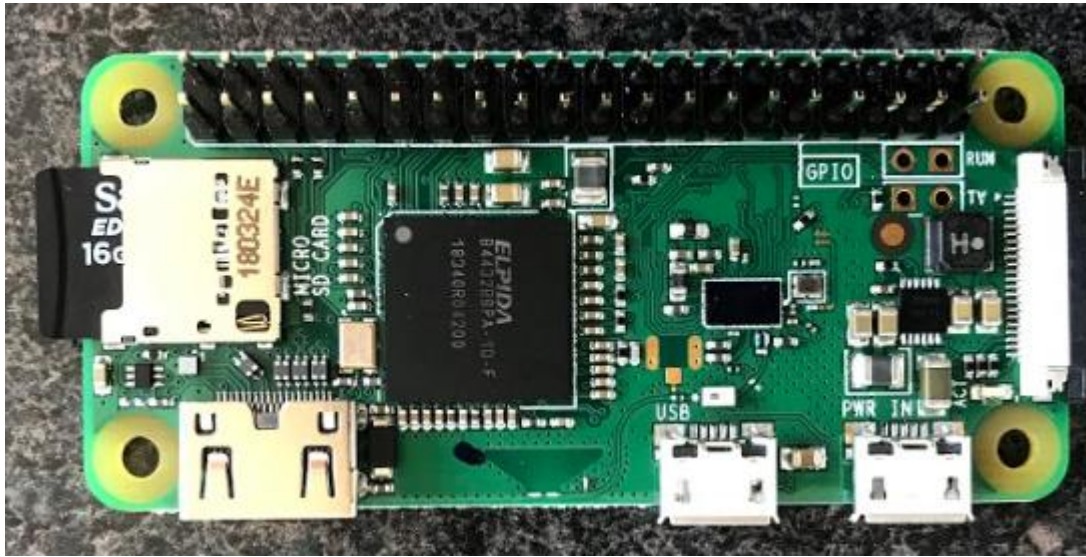
Figure 4-1: A photograph of a Raspberry Pi Zero (RPZ). This is the same RPZ used to build the mote for our prototype system.
