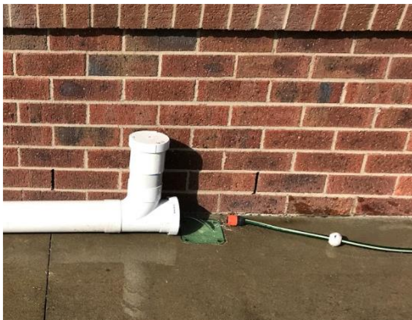
Figure 4-21: Water being drained from the test bed by removing the hose. Consequentially, the water level in the tall pipe dropped quickly and the float switch's contacts came apart. This simulates a surcharge ceasing, likely from a blockage no longer being present or from natural fluctuations in a partial blockage.
