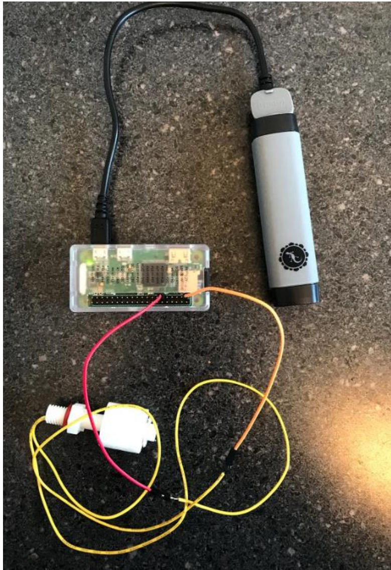
Figure 4-4: Our prototype mote. The Raspberry Pi Zero (RPZ) can be seen in the centre of the image, protected by a clear case. The float switch is connected to the device through the GPIO pins and can be seen at the bottom left-hand side of the image. Finally, the battery we utilised can be seen to the right of the RPZ, where it connects to the Micro USB power port.
