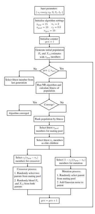
Fig. 2. Flowchart for hybrid algorithm
