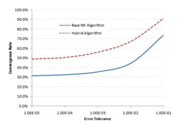
Fig. 4. Convergence rate versus error tolerance plot for NEMA motors
