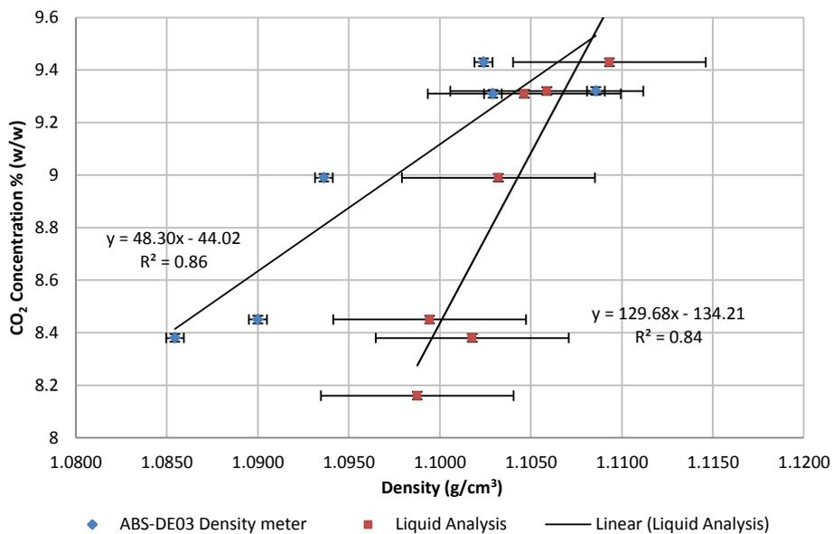
Figure 5 Comparison of steady state density measurements from the density meter ABS-DE03 (blue ♦) and liquid analysis (red ■) plotted with CO<sub>2</sub> concentration % (w/w). Note liquid analysis measurements are conducted as duplicates and the error bars shown are standard errors for the measurements
