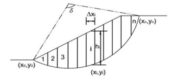
Fig. 1. Terms used to describe slip surface geometry.
