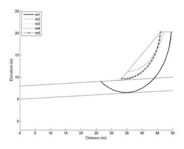
Fig. 4. Representative probabilistic slip surfaces detected by LIPS.
