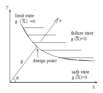
Fig. 2. Hasofer Lind reliability index shown graphically as the minimum distance from the origin to the limit state surface in a reduced normal space.
