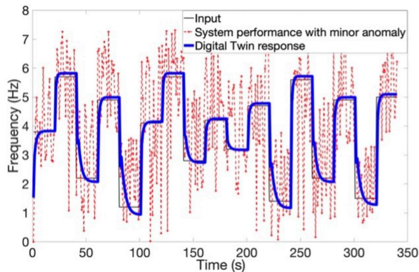
Fig. 16. ICS operation with minor anomaly instances
