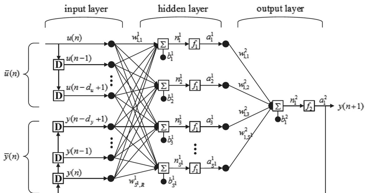
Fig. 3. illustrates the configuration of a NARX [54]
