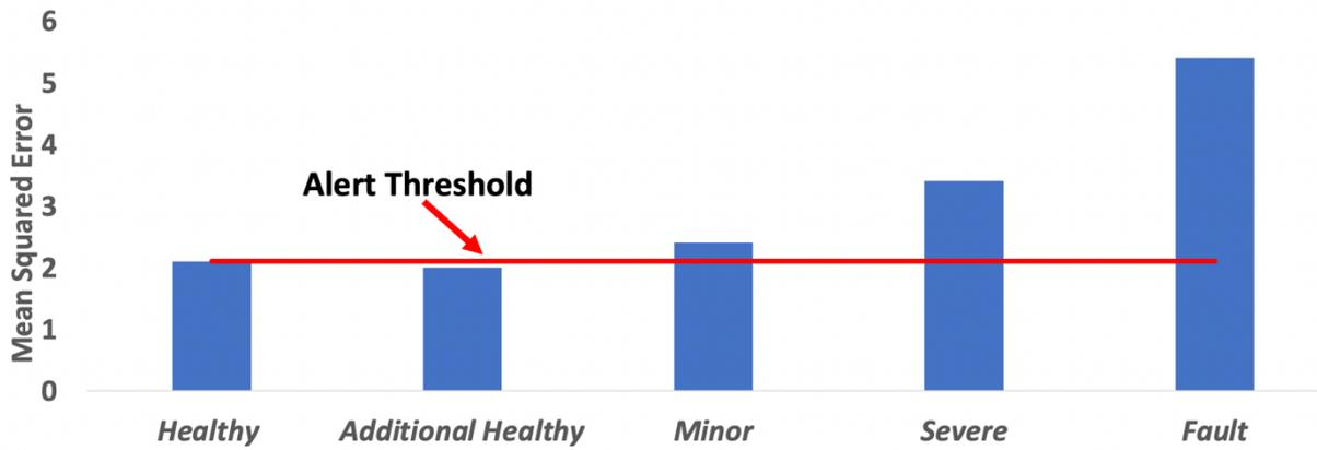
Fig. 20. DT Anomaly Detection, Quantification, and False Positive Mitigation
