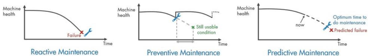
*Fig. 2. Different maintenance approaches [ Ref: MATLAB-
